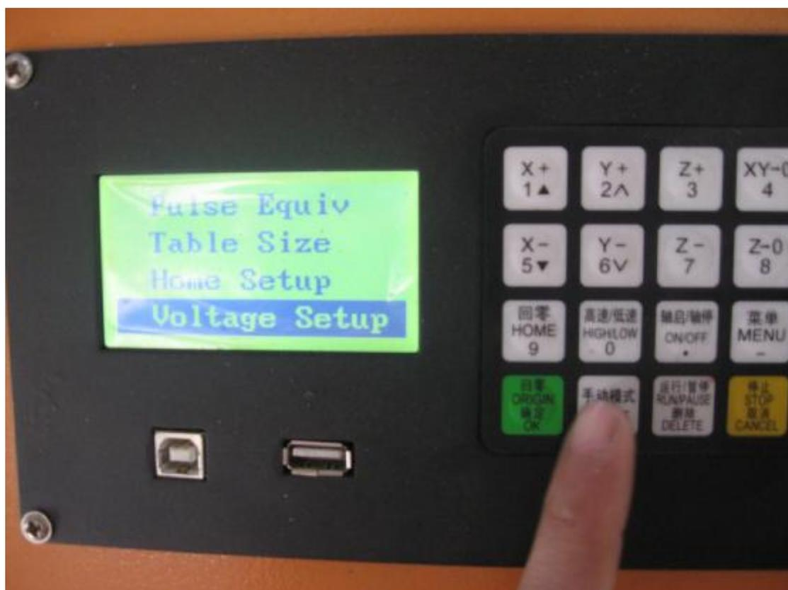
*SL1290 with step motor, parameters setting*
