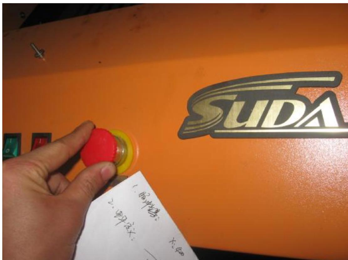
Stop the laser machine for a while, and start the laser machine again.
