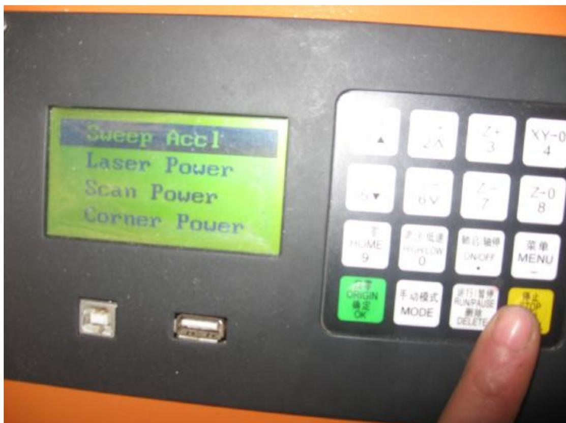
*SL1290 with step motor, parameters setting*
